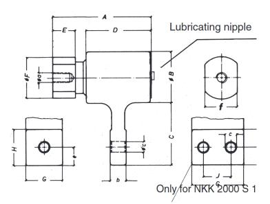
The use of an electronically controlled grease cup is recommended
