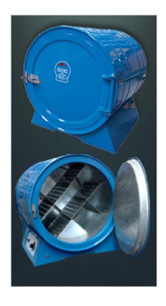
Welding electrodes should be stored in a heated enclosure to insure optimum performance. The coatings on electrodes will absorb moisture and this moisture will affect the ability of the electrode to produce a quality weld. Properly stored electrodes reduce the chances of weld porosity or cracking.
