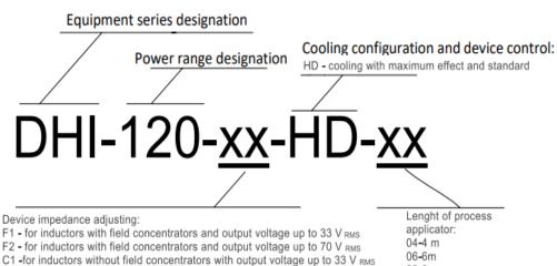
C2 -for inductors without field concentrators with output voltage up to 70 V RMS B1 - for soldering and brazing inductors with an output voltage up to 33 V RMS
